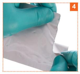
■ Tear the aluminium envelope open at the notch.Once the device has been taken out of the envelope its stability is of short duration, especially in a humid environment.
