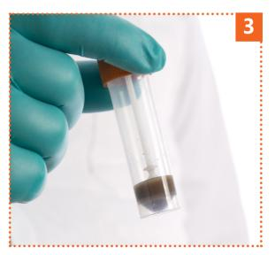
■ Dilute the sample with the liquid contained in the bottle. Homogenize well, taking care to prevent foam formation.
